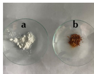
Figure 4 The color changes of the amoxicillin-lactose powder sample from the first day (a) to the fourth week (b) at 60°C
